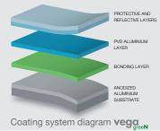
The coating parameters of the **vegg**, layers system are redefined (see below) to provide a strong shift of the maximum spectral reflectance to the orange and red zones most important for photosynthesis while maintaining high reflectance in the full visible light spectrum.
