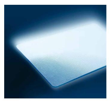
The LGP decouples light which is fed into the sheet from the sides across the surface area by the integrated prismatic optics. The optical structure is not acting as a diffusor but uses reflection and refraction of the microprisms. The direct portion of the light is usually also de-glared.
