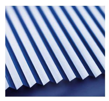
The LDP is another variation of our linear structures. This product offers smooth and highly efficient de-glaring capabilities along the main axis of the sheet. Numerically optimised pyramidal structures with sharp edge radii are ideal for high-precision light guiding applications and are being used frequently in thin luminaire fixtures.
