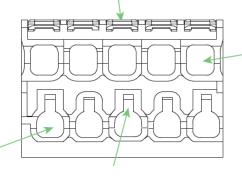
release opening for lower wires
